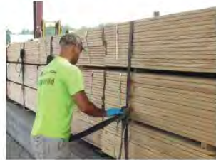
Figure 8-1. The charge is strapped to trams to keep it in place during treatment.
