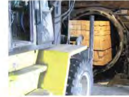
Figure 8-2. Using a forklift to push the charge into the cylinder for treatment.
