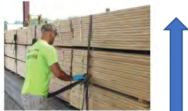
Figure 8-1. The charge is strapped to trams to keep it in place during treatment.
